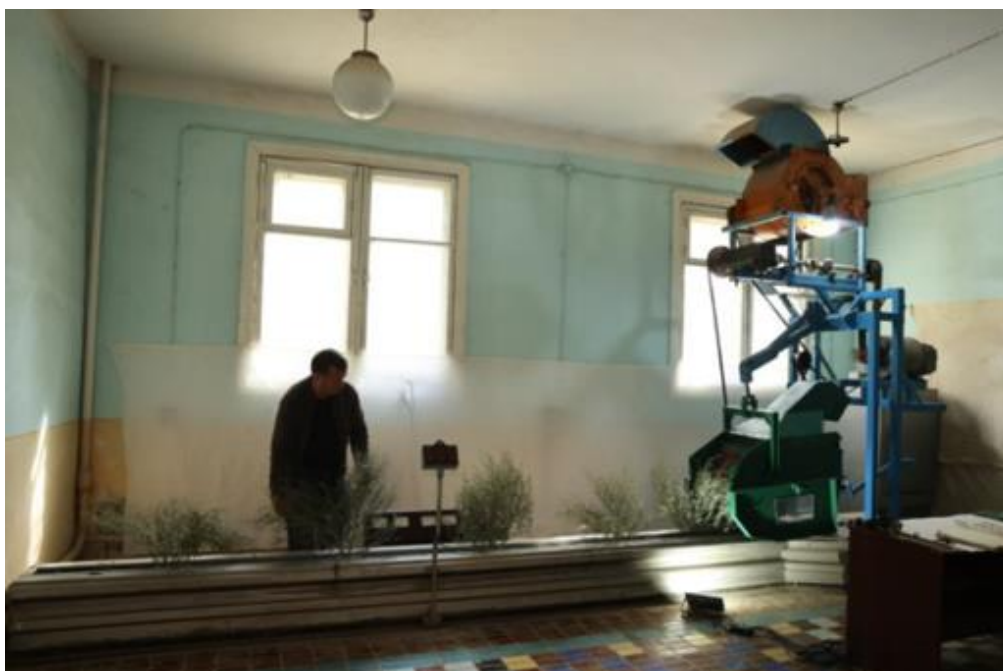
Fig. 1. Laboratory stand for determining the degree of stem splitting.
